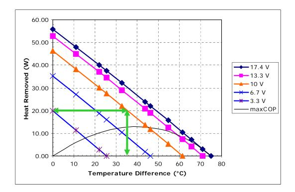
If you know the amount of heat load you need to remove and the desired cold-side temperature, you can determine what input voltage is required. Suppose you need to remove 20 W of heat at 15 °C and assume for now that the hot side of the module is at 50 °C. The temperature difference is then 50 - 15 = 35 °C. Therefore, the module would need a 10 V input.
