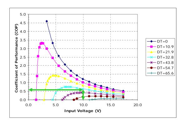
As with the heat removed in our current example, we have also already determined that the coefficient of performance (COP) is 0.6 [20 W of cooling divided by (10 V x 3.3 A) power input, 20/33 = 0.6]. However, this graph provides a visual indication of how far off of the maximum COP that the operating point is.
