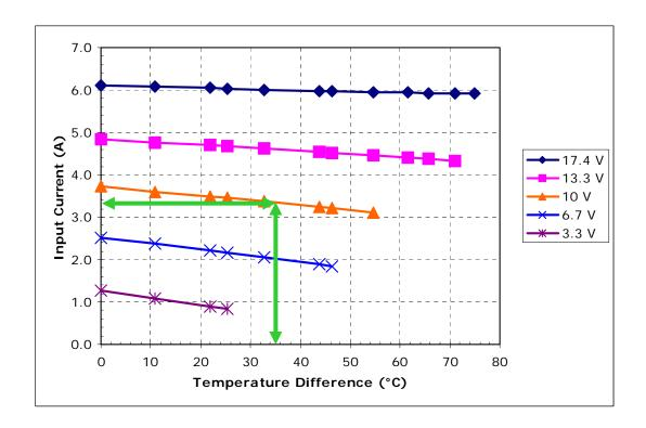
Once you know the input voltage, you can then determine what the steady-state current draw the module will have. In the example, a vertical line is drawn from the "Temperature Difference" axis until it intersects the graphed line representing the input voltage. Then draw a horizontal line from the intersection to "Input Current" axis to determine the current draw.
