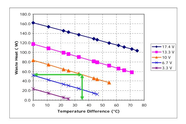
With our current example, we have actually already determined that the waste heat is 53 W (20 W of cooling plus 10 V x 3.3 A power input = 53 W). However, if you already knew the thermal resistance of your heat sink but did not know how much heat you could remove from the cold side, you could use this graph as your starting point.
