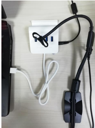
Use a powered USB 3.0 hub
